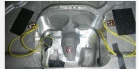
▲ Strain gauges for testing after HT
