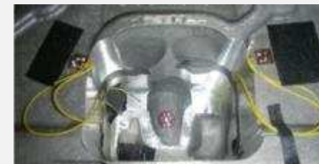
▲ Strain gauges for testing after HT
