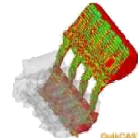
▲ Tilted gravity filling (QuikCast)
