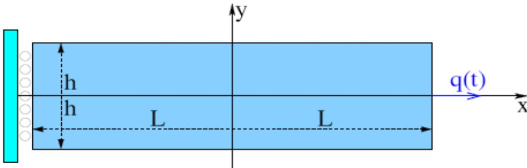
$$\begin{aligned} u_x(L, y) &= q(t) & u_x(-L, y) &= 0 & T_x(x, \pm h) &= 0 \\ T_y(L, y) &= 0 & T_y(-L, y) &= 0 & T_y(x, \pm h) &= 0 \end{aligned}$$
